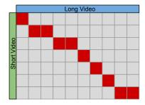
Fig. 1: The standard Dynamic Time Warping algorithm aligns all frames of both videos. Red squares represent aligned video frames.
